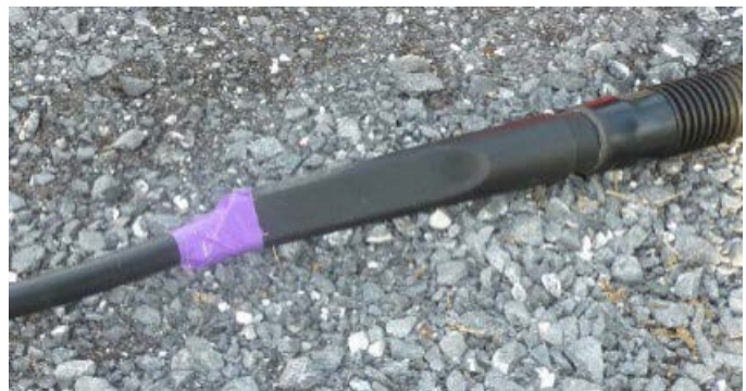
Figure 6: Tubing (left) taped to a shop vacuum crevice tool
