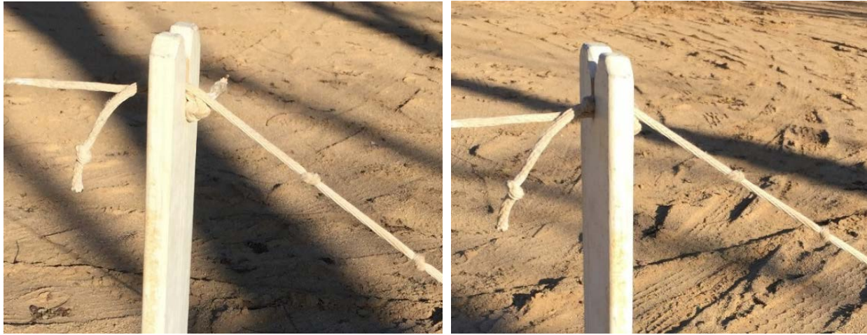
Figure 12: Counter-tilt upright, showing counter-tilt rope (to the left) and the hold down rope (to the right), with the hold down rope tightened to the 2 nd knot.
