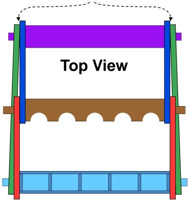
After cutting all the holes and assembling the rack, mark the sides of each outer board along the tenons so you know where the pegs need to go.
